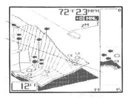
Bottom Lock is a function of zoom, except the depth adjustment is controlled automatically to view the area immediately above the bottom. This is especially useful if you are looking for structure or minor variations in terrain in areas of relatively flat bottom terrain. To enable Bottom Lock, press ENTER until the "BL" is highlighted. The zoom range will be controlled by the current depth range, as in Zoom, and will be indicated on the Zoom menu.
